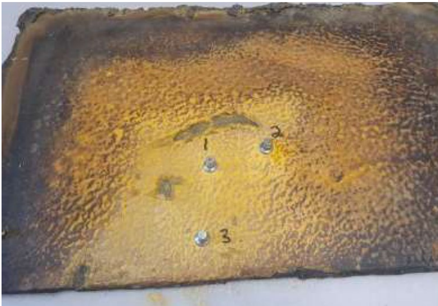
Figure 5-2 Carbon steel sample coated retrieved from atmospheric zone of Ekofisk 2/4A when structure was decommissioned in 2020, ref. /5/. Edges are damaged due to cutting of the sample and center of the sample was used for further examined.
