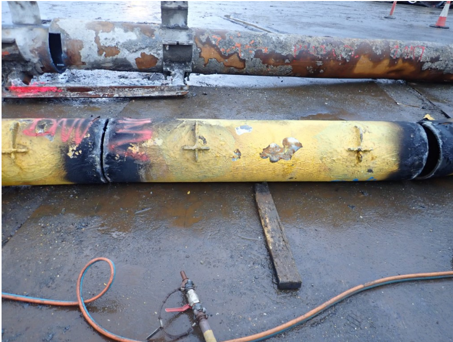
Figure 6-6 2 m length of brace from EL +20' further examined at DNV laboratory in Bergen, ref. /17/.
